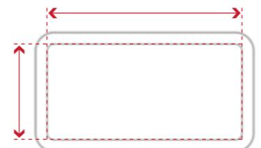
\*Network access chamber sections are measured by the inside measurement of the chamber ring section and this is referred to as the clear opening.
